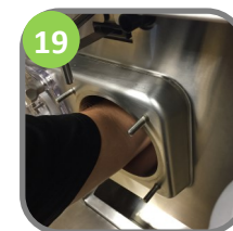
Thoroughly Clean Rear of Cylinder
