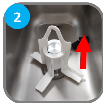
Remove Hopper Agitator (Optional)
