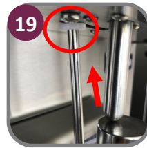
With tapered end down, install torque arm up through the sensor pin hole under the overhead and then down into the torque assembly; torque arm should move freely back and forth.
