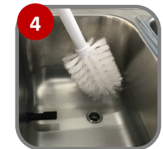
Scrub Hopper Sides and Bottom
