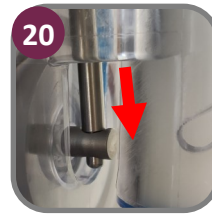
With tapered end down, install torque arm up through the sensor pin hole under the overhead and then down into the torque assembly; torque arm should move freely back and forth.
