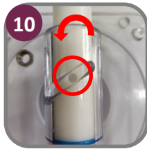
Make Sure the Draw Handle Hole is Accessible
