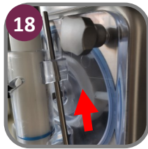
With tapered end down, install torque arm up through the sensor pin hole under the overhead and then down into the torque assembly; torque arm should move freely back and forth.
