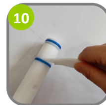
Remove Draw Valve O-Rings
